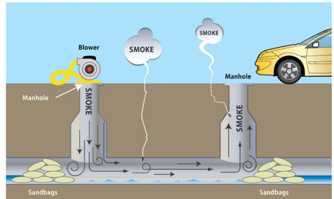
If there are defects in either the main sewer pipes or the private sewer laterals that serve individual homes and businesses, or if there are illegal cross-connections between the sewer and storm drain, smoke will rise to the surface and reveal these problems.
